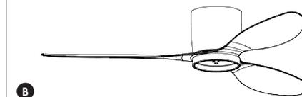
Unscrew the set screw. Attach the LED pan to the bottom of the fan by inserting the other two set screw into the corresponding slots. Rotate the unit, then secure the previous set screw by aligning it with the screw hole and the hole at the bottom of the fan. Finally, tighten the last two set screws to secure LED pan.
